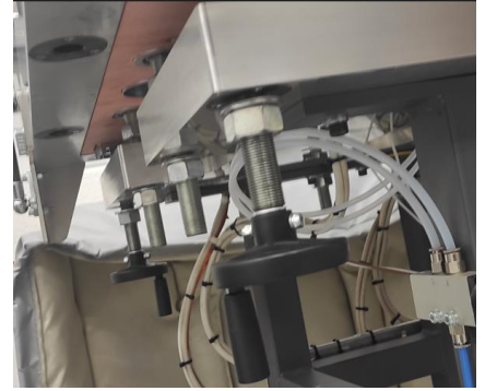
Figure 19 Locking nuts under mould cavity.
