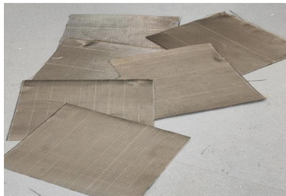
Figure 16 2D structure, six carbon fibre sheets
