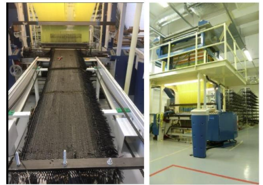
Figure 8 Jacquard Controlled Weaving Loom located in NIACE (UKRI, 2023)
