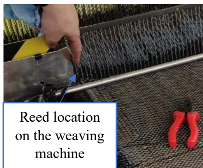
Figure 11 Reed location on the Jacquard Controlled weaving loom.
