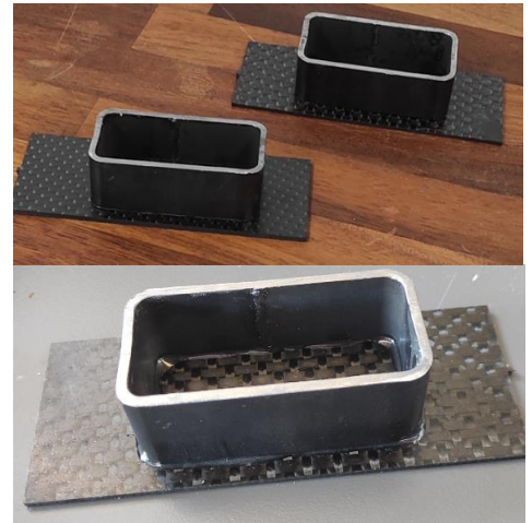
Figure 35 80X40X20mm box section with composite specimens
