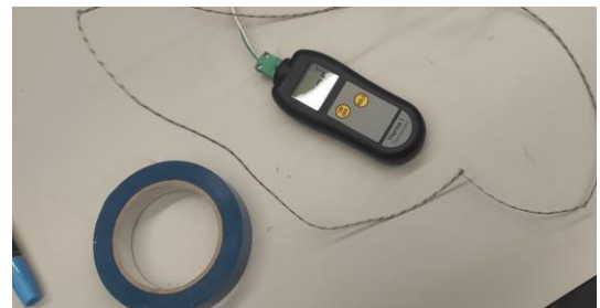
Figure 32 High temperature tape and type K thermocouple and digital read out meter.
