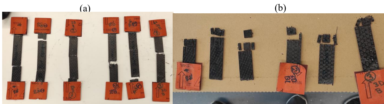
Figure 38 Random selection of tensile test specimens (a) and CT specimen tabs (b)
