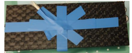
Figure 36 Thermocouple, composite attachment
