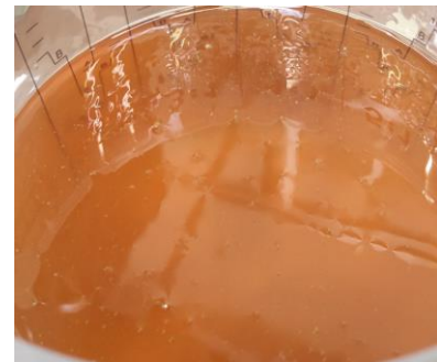
Figure 26 Illustration of air bubbles formed when mixing.
