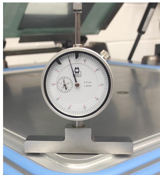
Figure 18 Zeroing depth gauge using cavity corners.
