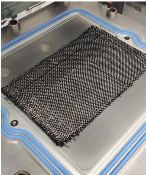
Figure 23 Placing fabric on the mould face ensuring seal is free from interference.
