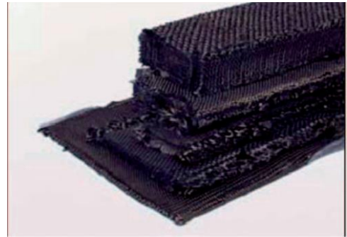
Figure 6 Comparison of 2D laminate and woven 3D preform (X. Chen et al., 2011)
