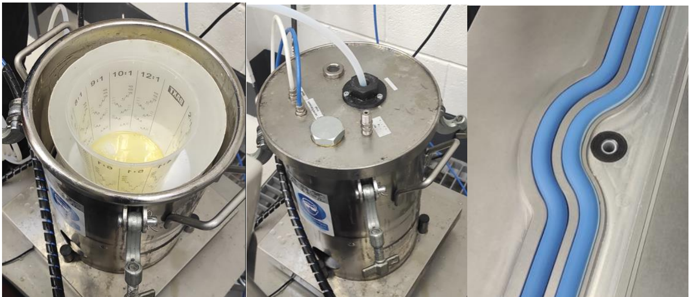
Figure 20 Resin pipe installation from resin vacuum pot to mould.
